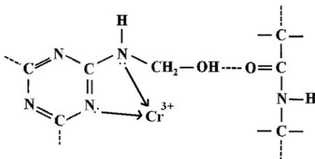
Fig. 3. The possible interaction of melamine with collagen chains through chelation involving Cr<sup>3+</sup> of chrome complex and H-bonding
