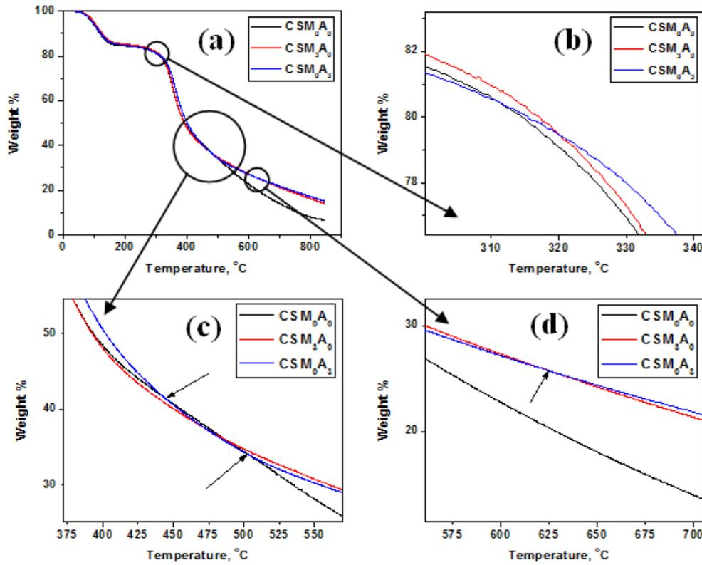
Fig. 2. TGA results of the samples CSM<sub>0</sub>A<sub>0</sub>, CSM<sub>3</sub>A<sub>0</sub>, and CSM<sub>0</sub>A<sub>3</sub>
