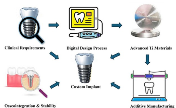
Figure 1. Digital workflow for customized dental implant fabrication, illustrating the integration of clinical diagnosis, digital planning, CAD, material selection, additive/ subtractive manufacturing, and final implant placement
